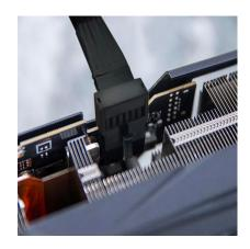
12VHPWR native cable with 90 degree connector provides easy installation.
